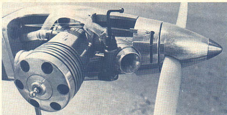
Side-mounted engine keeps exhaust away from Seebig timer. Spacer between pan and firewall required to mount the gear. Prop brake is a must with 7-sec. motor runs—eliminates run-down affect. Brake is modification of Brodersen brake. Below: Auto-stab detail; stab is held down against fuselage by auto-stab line in the power mode. Right: Here the auto-stab dethermalizer line has been released, allowing stab bracket and "ail" to pop up to the DT position.
