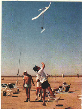
F1B World Champion Alexander Andriukov gives his AA 26 the high heave. Delayed prop release adds 20 or more feet of extra altitude—quite valuable in flyoffs, or to max in marginal air.
