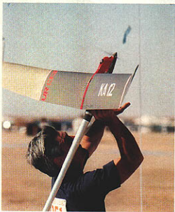
The Ukrainian Kirilenko, 15th in F1C. Clean model had gold anodized wing sheathing, said to add extra torsional rigidity due to its enhanced tempering.
