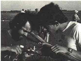
Adjusting the propeller brake on his Stromboli is Michel Iribarne of France. Notice the angled mounting of his engine.
