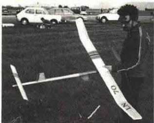
Norwegian accent on the Scandinavian Wakefield, as shown by Ole Torgersen. High aspect ratio wing, a long fuselage and small tail surfaces.
