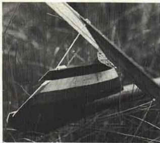
This simple tailplane mounting on his T-tail Wakefield was used by Poczobut of Poland. Note the tab on the pylon/fin beneath stabilizer.
